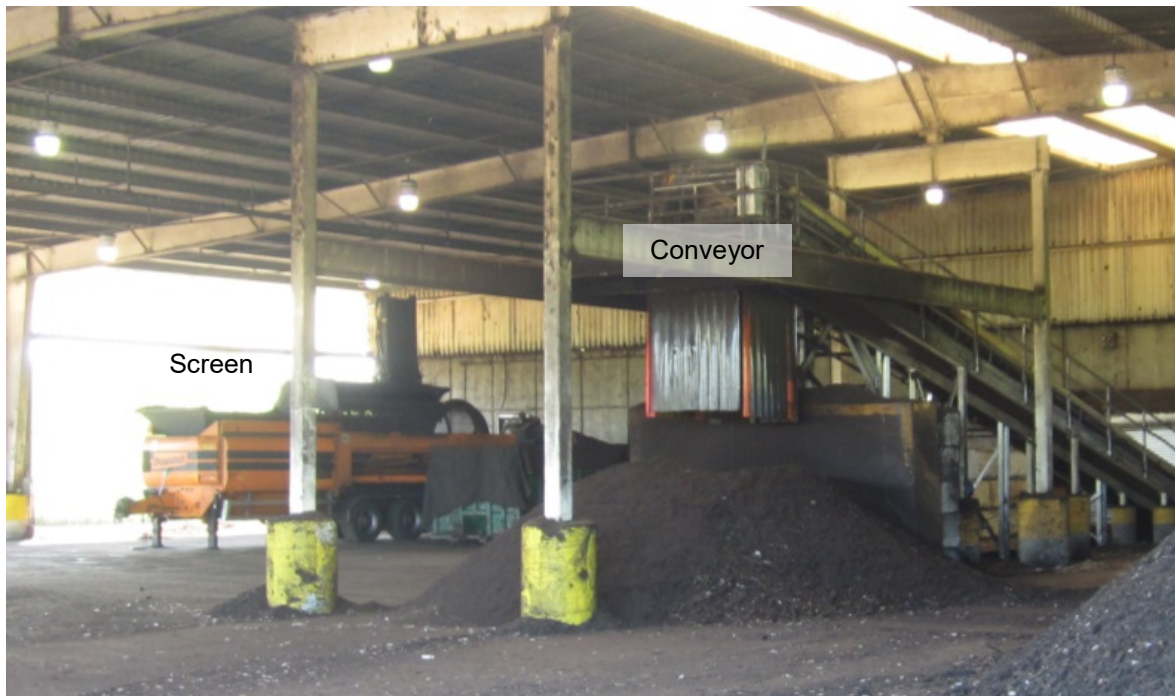
Figure 2-5: Screening Equipment Location Relative to Conveyor
