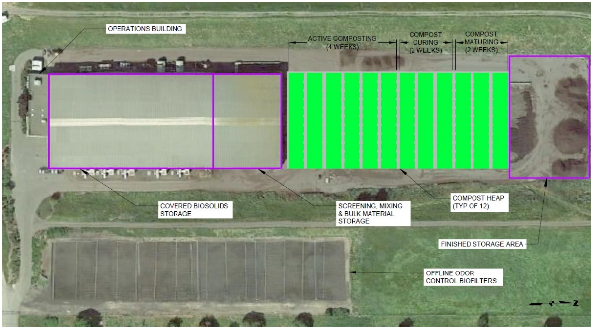
Figure 6-4 Covered Aerated Static Pile Site Layout
