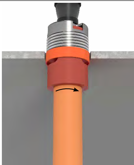
Figure 6: Using the Sprinkler Wrench
