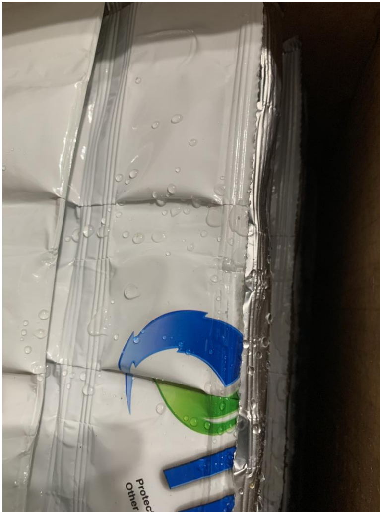
Figure 37: PCM mat with water accumulation at the BSRL
