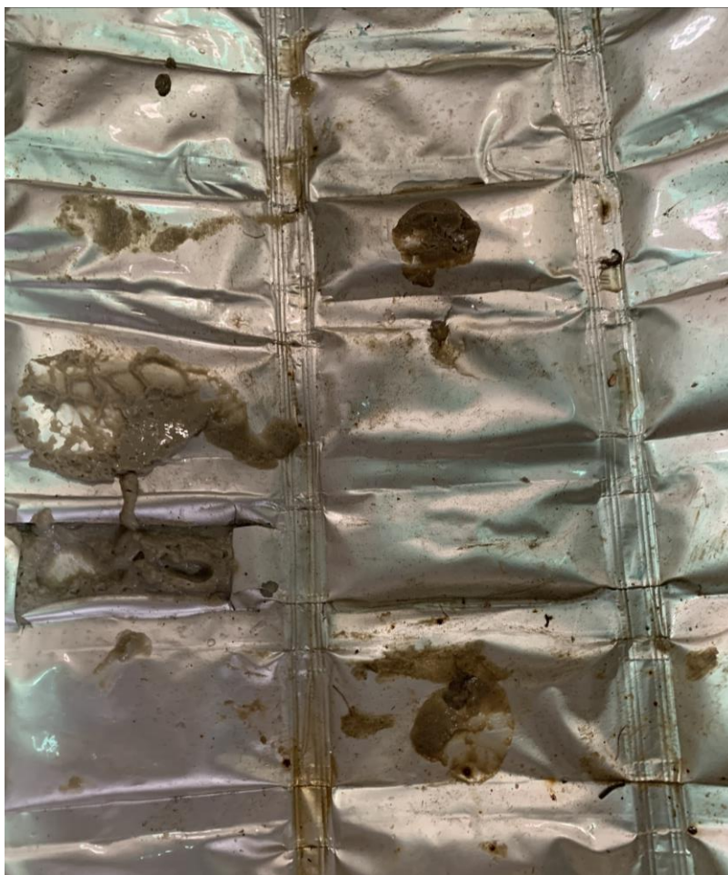
Figure 35: PCM mat with multiple leaks near scuff marks from Site 54
