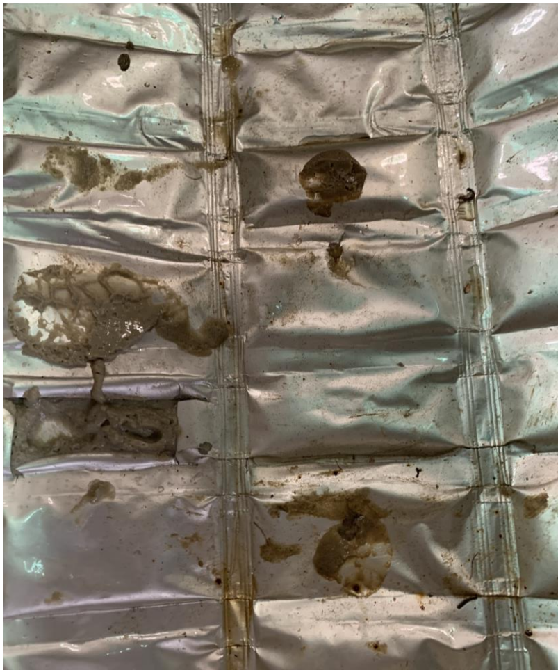
Figure ES-4: PCM mat with multiple leaks near scuff marks from Site 54
