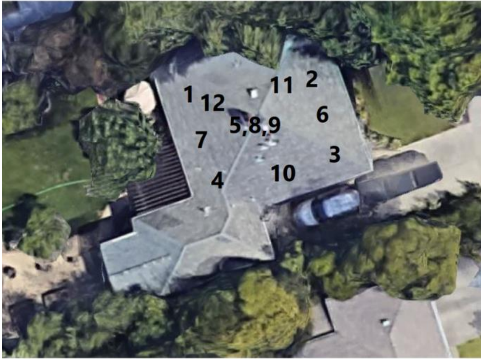
Figure 16: Site 54 Sensor Locations (Pre-Monitoring)
