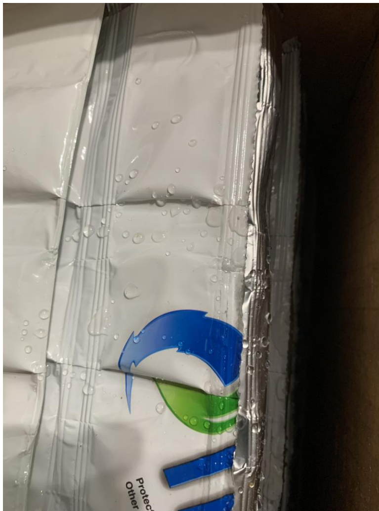
Figure ES-5: PCM mat with water accumulation
