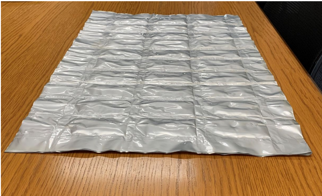
Figure 2. PCM mat used for residential attic applications. Image credit: Bob Hendron
